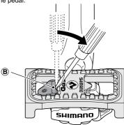
$\textbf{4.} \ \, \text{Turn the adjustment bolt on the pedal to adjust the spring tension to the strongest setting.}$
