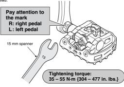
A 6 mm Allen key cannot provide a sufficient tightening torque. Always be sure to use a 15 mm spanner
