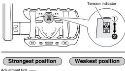
Spring plate If the tension indicator is at the strongest or the weakest position, do not turn the adjustment bolt any further.
