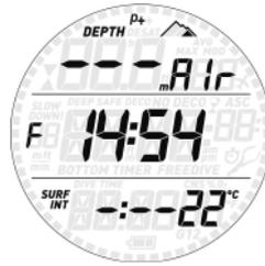
The pre-dive display shows p factor and altitude settings, time of day, surface interval and temperature. If Nitrox is set, it will show the O<sub>2</sub> percentage and the corresponding MOD. A small S or F to the left of the middle row indicates the water type.
