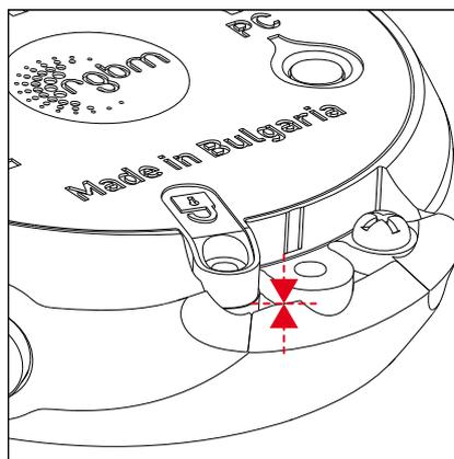
i) Keep the cover pressed onto the watch case while hand tightening the two screws. Don't use excessive force while tightening. Ideal torque is 12 N cm / 17 oz-in.
