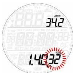
Once inside this menu, press either button to change the  $O_2$  and observe how this affects the maximum operating depth (MOD). Then press and hold the upper button to move on to the  $ppO_2$ max and use either button to change the value, again noticing how this affects the MOD. Press and hold the upper button again to save the setting.
