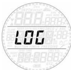
Smart can record the profiles of approximately 35 hours of diving, at a sampling rate of 5 seconds. The information can be transferred using the optional USB clip to PC via the Dive Organizer software or to a Mac via the Divers'
