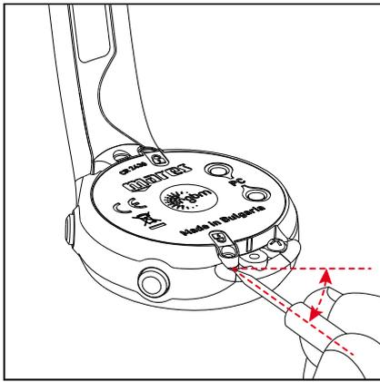
d) Remove the cover then remove the o-ring. Discard the o-ring.
