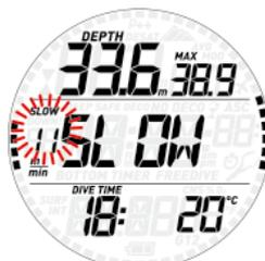
If the ascent rate exceeds 12m/min / 40ft/min at a depth below 12m / 40ft, **SLOW DOWN!** appears and the speed value blinks. If a speed in excess of 12m/min / 40ft/min is maintained for two thirds or more of the depth at which the alarm was first triggered, Smart considers it a dive violation and the display will show the steady **SLOW DOWN!** symbol.
