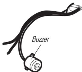
Secure the buzzer to a nearby wire bundle using the cable ties (included).
