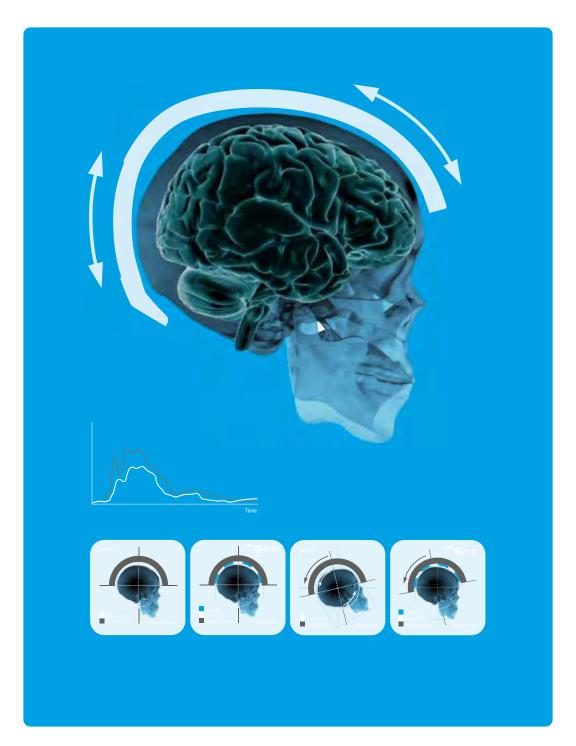
POC's patent pending rotational impact protection system, SPIN (Shearing Pad Inside), is an evolution in head and brain protection. Through the use of innovative and unique pads inside a helmet it is possible to reduce the amount of force transmitted to a user's head and brain in the event of an oblique impact.
